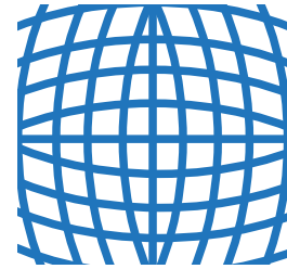
Barrel distortion Negative radial displacement
